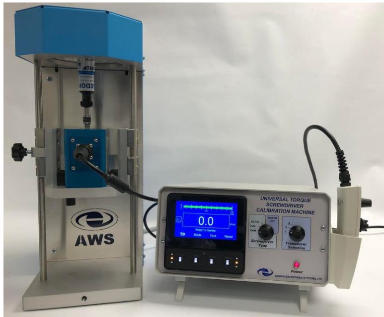
Photo above shows a UTSCM with Control Box, Handheld Controller, and an Intelligent Inline Torque Transducer.
