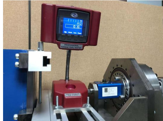
Torque Tester Extension with fittings for horizontal mount Torque Testers. AWS PTTT shown as device under test. (Sold separately)
