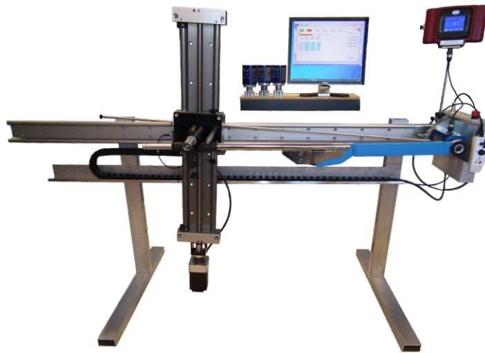
Photo above shows a UTWCM with AWS Intelligent Inline Torque Transducers, Professional Transducer Display, and Laptop/Computer running ADMS Kepler 4 Software for Calibration & Conformity to ISO 6789:2017 Parts 1 and 2.
