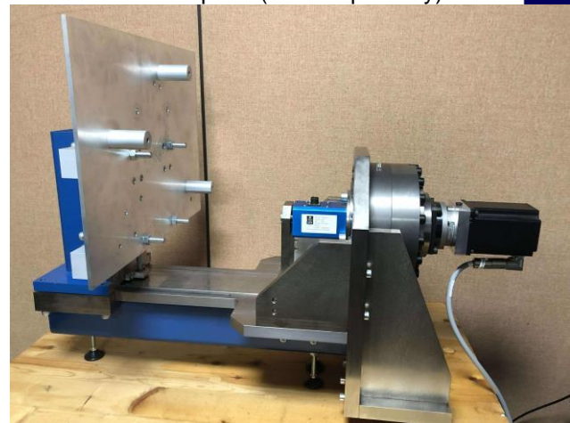
UTCM with Tool Tester Extension and Vertical Mounted Torque Tester fittings.
