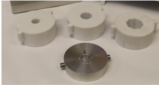
Photo above shows various AWS solid torque screwdriver handle adapters.
