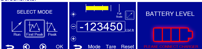
Left: Graphical mode selection. Centre: Reading screen showing mode/units selected and analogue bar graph. Right: Battery level warning
