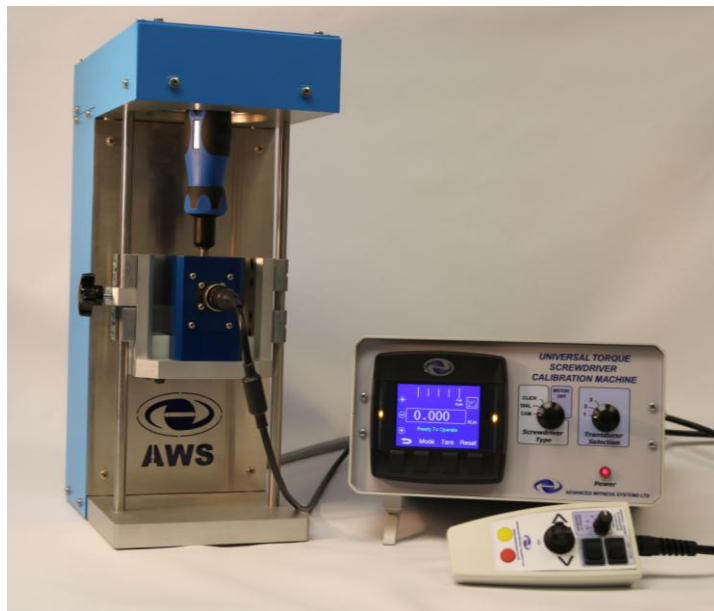
Photo above shows a UTSCM with Control Box, Handheld Controller, and an Intelligent Inline Torque Transducer.
