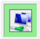
This icon on the top right of the “**Readings**” screens indicates that the device is connected.
